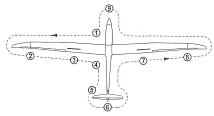
When walking around the "Duo Discus", check all surfaces for paint cracks, dents and unevenness.
