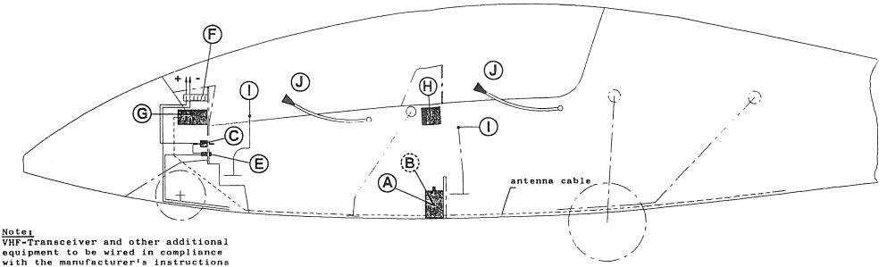
VHF-Transceiver and other additional equipment to be wired in compliance with the manufacturer's instructions and to be fused individually.
